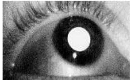
(d) Example of “bright pupil” (and corneal reflection) illuminated by infra-red light. Courtesy of LC Technologies, Fairfax, VA < http://www.eyegaze.com >. Reproduced with permission.
