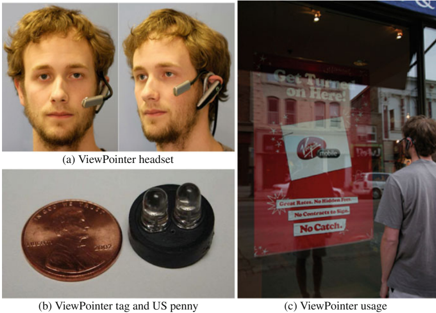
Fig. 24.4 ViewPointer headset, tag, and usage: a user looks at a poster augmented with an invisible ViewPointer URL tag mounted behind the poster's logo. From Smith et al. (2005) © 2005 ACM, Inc. Reprinted by permission
