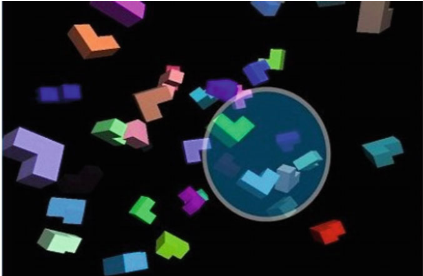
(a) Important collisions (e.g., those close to the viewer's fixation position) are processed first
