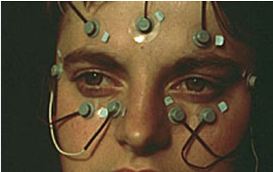
Fig. 5.1 Example of electro-oculography (EOG) eye movement measurement. Courtesy of Metro-Vision, Pénchenies, France ( http://www.metrovision.fr ). Reproduced with permission
