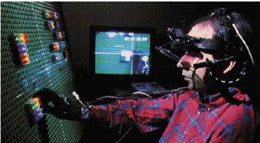
Fig. 21.8 Eye tracking in a natural pick-and-place task. Courtesy of Jeff Pelz, Visual Perception Laboratory, Carlson Center for Imaging Science, Rochester Institute of Technology http://www.cis.rit.edu/people/faculty/pelz/research/ASL_tracker.html . Reproduced with permission
