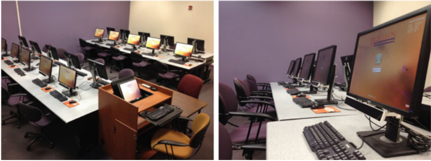
(a) Classroom with 20 Gazepoint trackers. (b) Close up of Gazepoint tracker mount.
